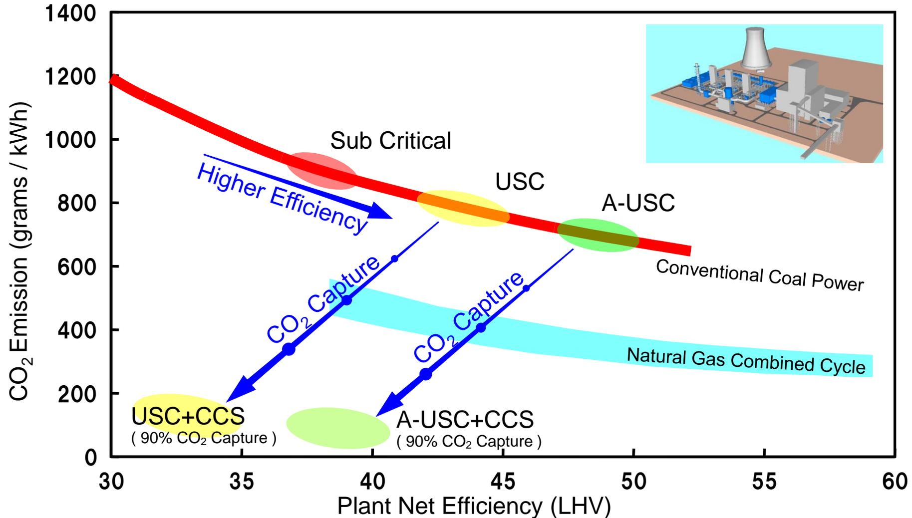
Substantial CO<sub>2</sub> reduction is realized by Integration and Optimization of both High efficiency Turbine Cycles and CCS technology
